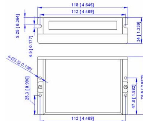
Figure 1: Mechanical specifications
