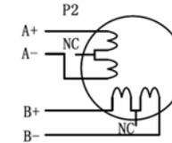
Figure 6: 6-lead motor full coil (higher torque) connections
