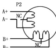
Figure 6: 6-lead motor full coil (higher torque) connections
