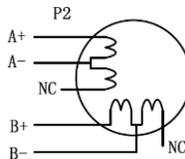
Figure 5: 6-lead motor half coil (higher speed) connections
