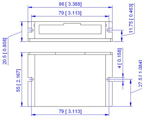
Figure 1: Mechanical specifications
