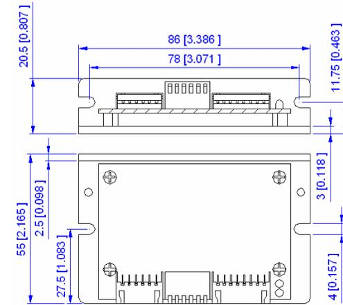
Figure 1: Mechanical specifications
